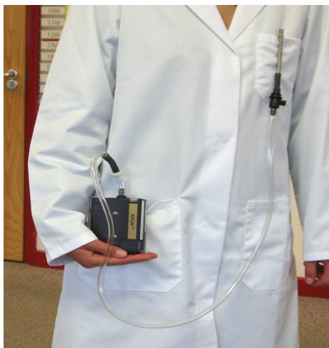
Fig 1. Pumped Sampling (Pump can be fitted to pocket or belt).
